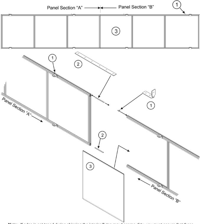
**Note:** If edge is not taped during shipping the interior flutes may become dirty, you must ensure that these flutes are cleaned before the poly glass panel is installed into the assembly.
