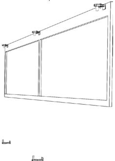
**5.** Prep your Nova-Lite panel with secondary cables by fastening them to the upper track clips (thimbles and cable clamps are used for the secondary installation). Note: that the Nova-Lite panel may be put into place resting on the bottom track brackets before you install the tracks. Please also read step 6 before proceeding.
