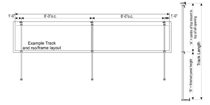
**3.** Establish track length from top bracket to the location where the bottom bracket is to be installed. The track length must allow the panel to open its full depth past the sill of the opening. This track length is Length "A" plus Length "B" plus ½" to equal track length.
