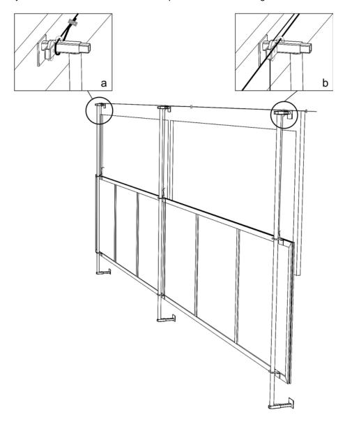
**9.** Position the panel flush with the top of the sill. With the main cable under tension the secondary cables may now be hooked up. (a) View of secondary cable hooked up to panel. (b) Please note that the thimbles and cable clamps or crimps must have been used to pre-install the secondary cables in step 5.
