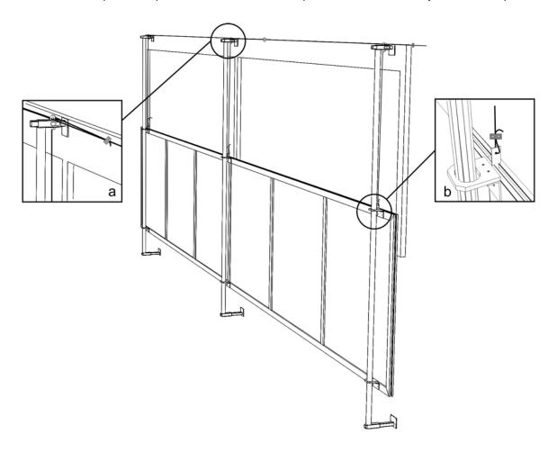
**Note:** Areas that require greater travel length or when end pulleys are near the end panel you will be required to install a double back pulley system as shown in these pictures.
