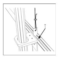
**12.** Position the panel ½ open and attach the bottom track guides to the face of the panel.
