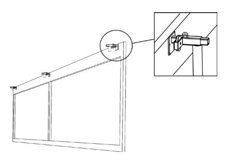
**Note:** Always remember to install two panel track support guides onto each track as shown in the middle figure below. This must be done when the track is installed. The smaller of the two supports is to be mounted to the top end of the track while the larger support is for the bottom.
